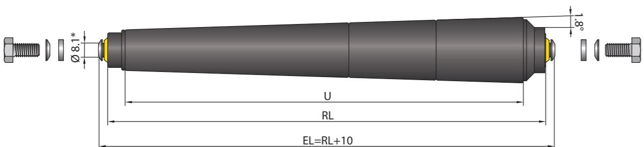
\* The recommended profile holes have a dimension of Ø 8.1 mm
